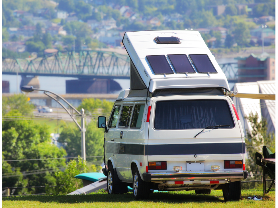
Figure 19. In recreational vehicles, PV panels can be used to supply electricity to dc powered devices and keep the battery charged.
